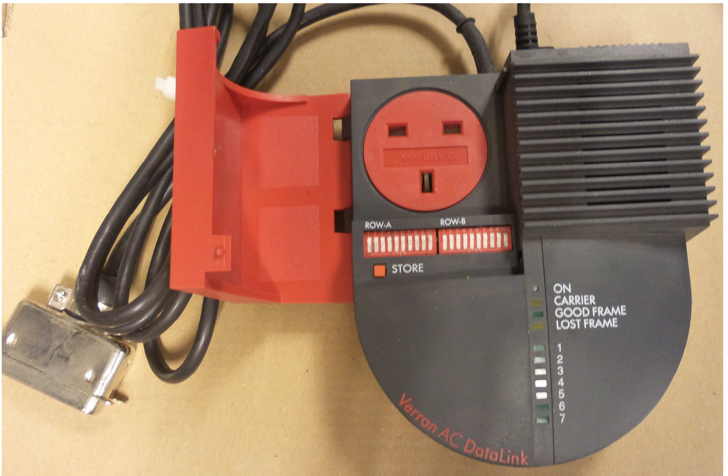
Figure 23: Verran frontend powerline printer/plotter sharing adapter S/N CAB 9003100257, top view
