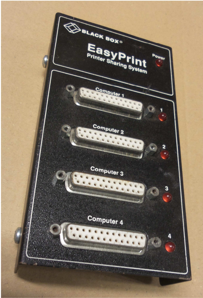
Figure 16: BlackBox EasyPrint backend powerline printer/plotter sharing adapter
