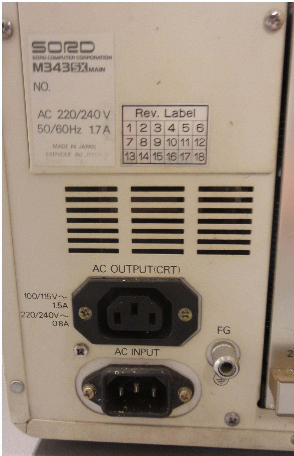
Figure 10: SORD M343SX manufacturing labels and mains AC input and output “M343SX No. AC 220/240V 50/60Hz 1.7A Made in Japan Fabrique au Japon”
