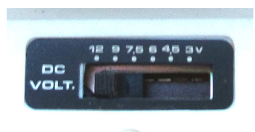
Figure 6: Linguaphone MR-L5 power supply unit (NB: set to 12V) ROSS RE 551, 230/240V 50Hz, 3V / 4.5V / 6V / 7.5V / 9V / 12V DC 300mA, Complies with BS 415 & BS 1363
