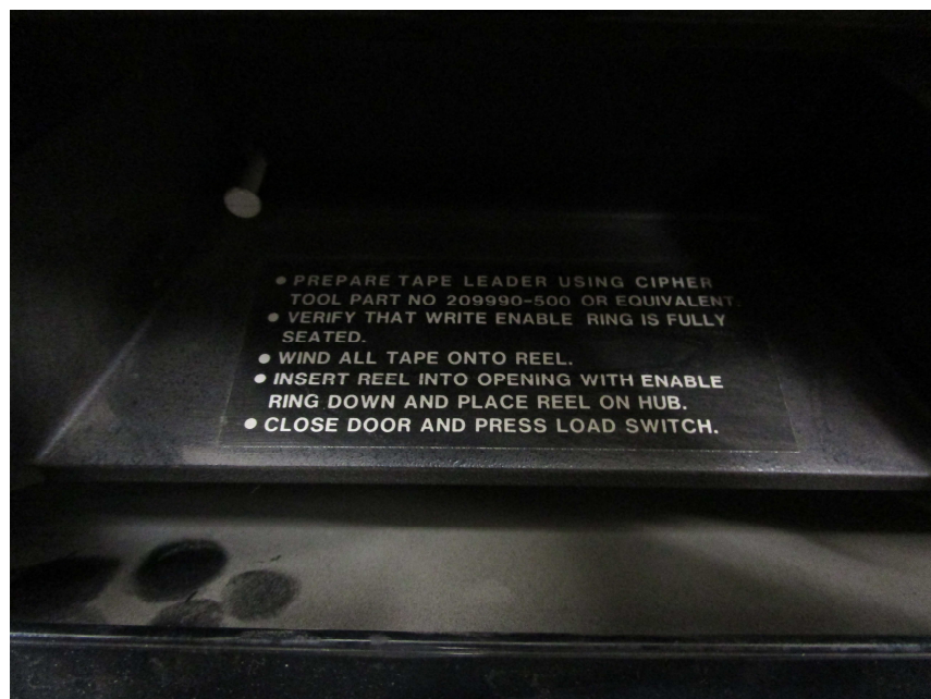
Figure 4: Cipher F880 tape loading instructions
