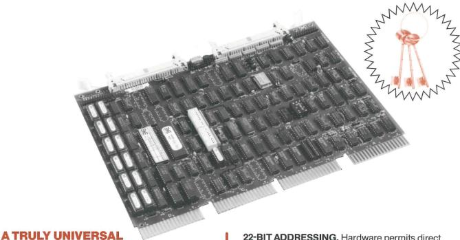
The TC02 has DEC™ TS11 diagnostic/software transparency and standard operating system support across the MicroVAX™I and II, MicroPDP™ and LSI-11™ CPU lines. The TC02 also handles industry-standard half-inch tape transports — conventional start/stop, streaming, and the new generation of GCR units. Compactly packaged on a single quad-height board with low power consumption, the TC02 is backed by worldwide support and the EMULEX brand of quality.
