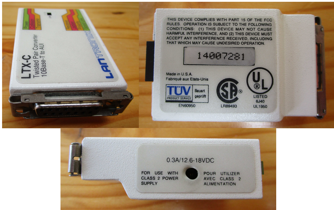
Figure 15: Lantronix LTX-C 10BASE-T to AUI transceiver S/N: 14007281
