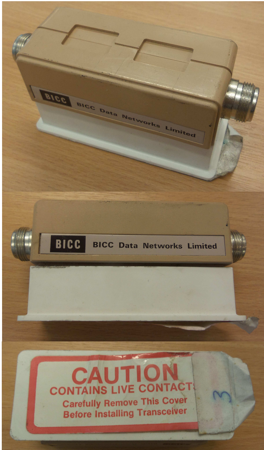
Figure 5: BICC Thickwire adapter, separated from Ethernet transceiver 'Caution' label covers contacts for mating with transceiver
