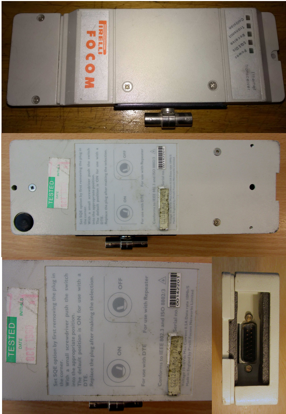
Figure 10: Piirelli FOCOM Thinwire to AUI transceiver P/N:522124A Mod 1/A12 , S/N: 00142201
