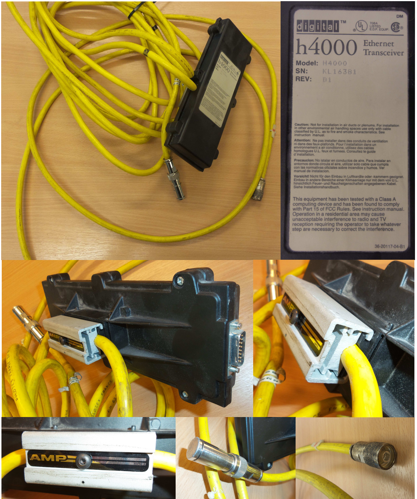
Figure 3: DEC H4000 first-generation Thickwire to AUI transceiver coupled to Thickwire coaxial cable Note light-gray Thickwire adapter mated with black Ethernet transceiver, and silver terminators at cable ends H4000 Rev.D1, S/N: KL 16381
