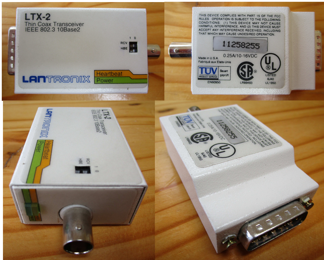
Figure 13: Lantronix LTX-2 Thinwire to AUI transceiver S/N: 11258255
