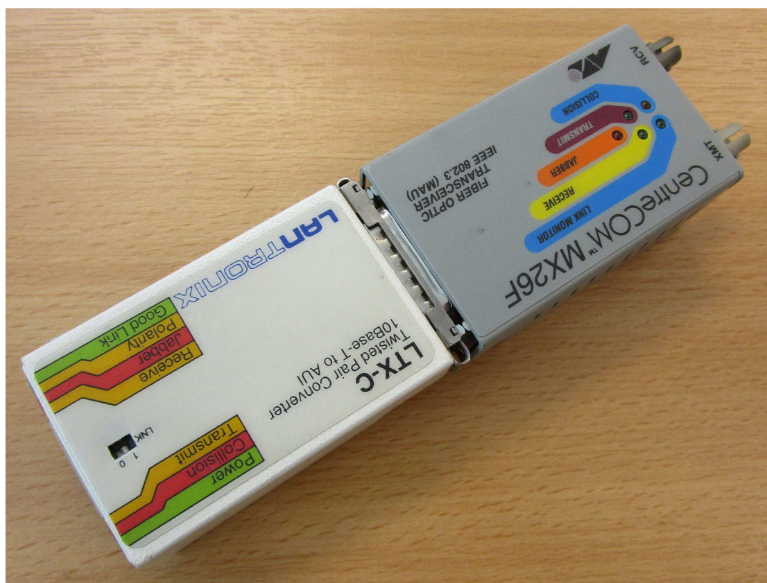
Figure 18: Lantronix LTX-C 10BASE-T and CentreCOM MX40F/ST 10BASE-FL to AUI transceivers coupled together to link 10BASE-T to optical fibre
