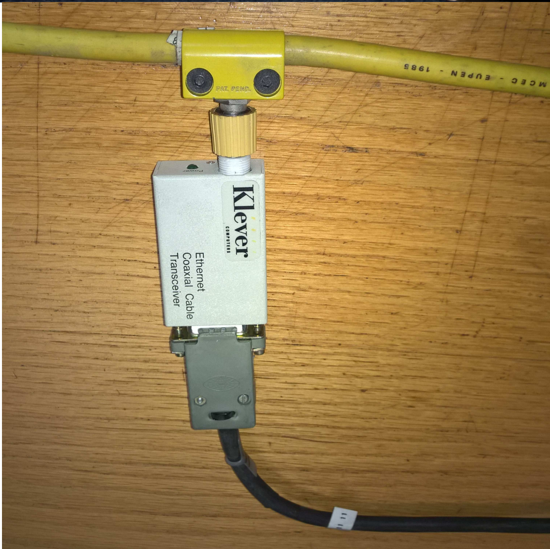
Figure 9: Klever Thickwire to AUI transceiver before and after attachment to 10BASE5 Ethernet coax cable (Klever transceiver mated to Thickwire adapter)
