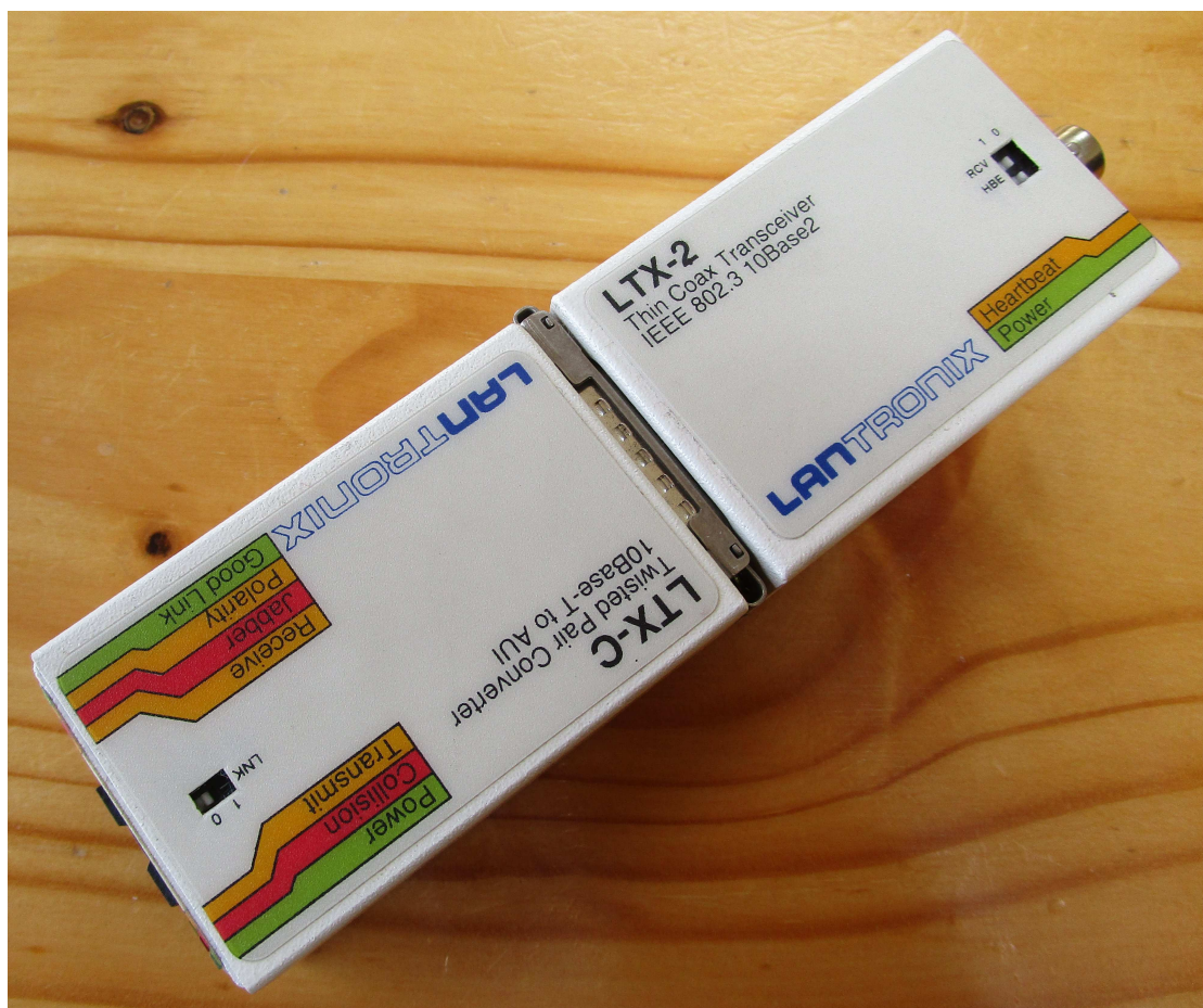
Figure 16: Lantronix LTX-C 10BASE-T and LTX-2 Thinwire to AUI transceivers coupled together to link 10BASE-T to Thinwire
