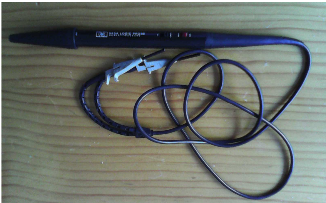
Figure 4: HP-545A Logic Probe front view, with cover on probe tip
