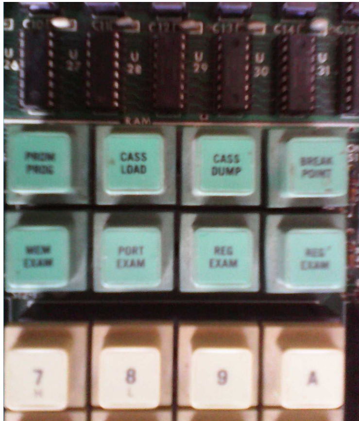
Figure 4: Zilog Z80 SDK Development Kit keyboard top closeup
