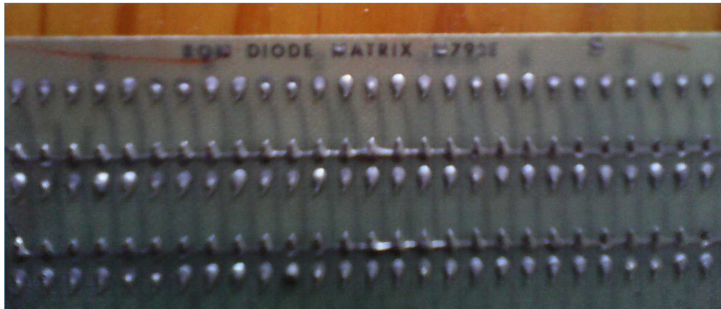
Figure 3: DEC M792E manufacturing label "ROM DIODE MATRIX 792E"
