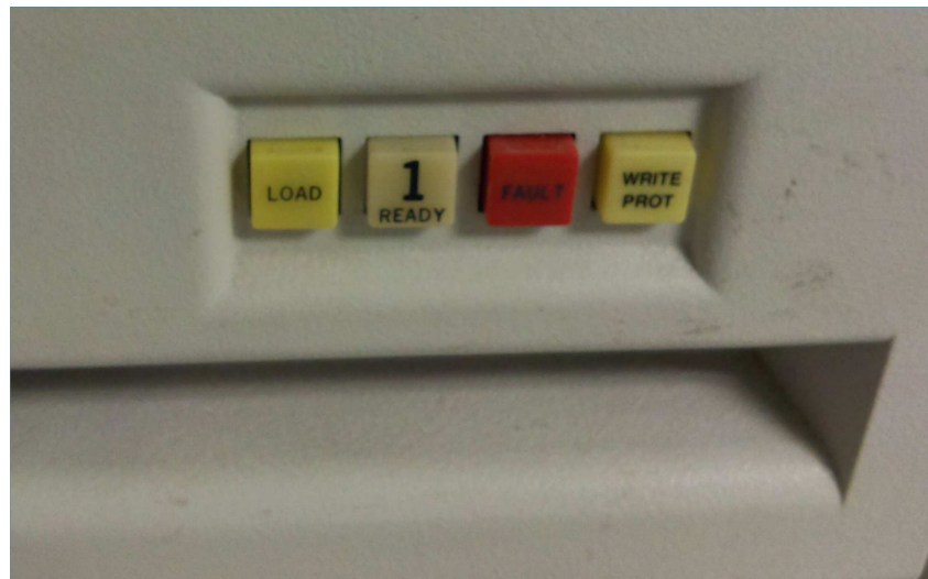
Figure 6: PDP 11/84 Disk Drive (2) control panel closeup
