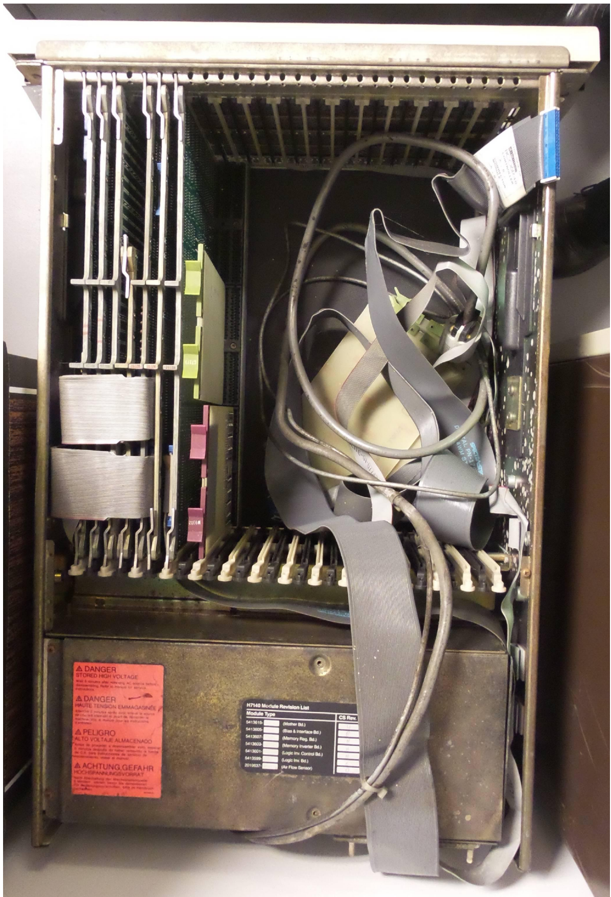
Figure 8: DEC PDP 11/24 CPU chassis, top view
