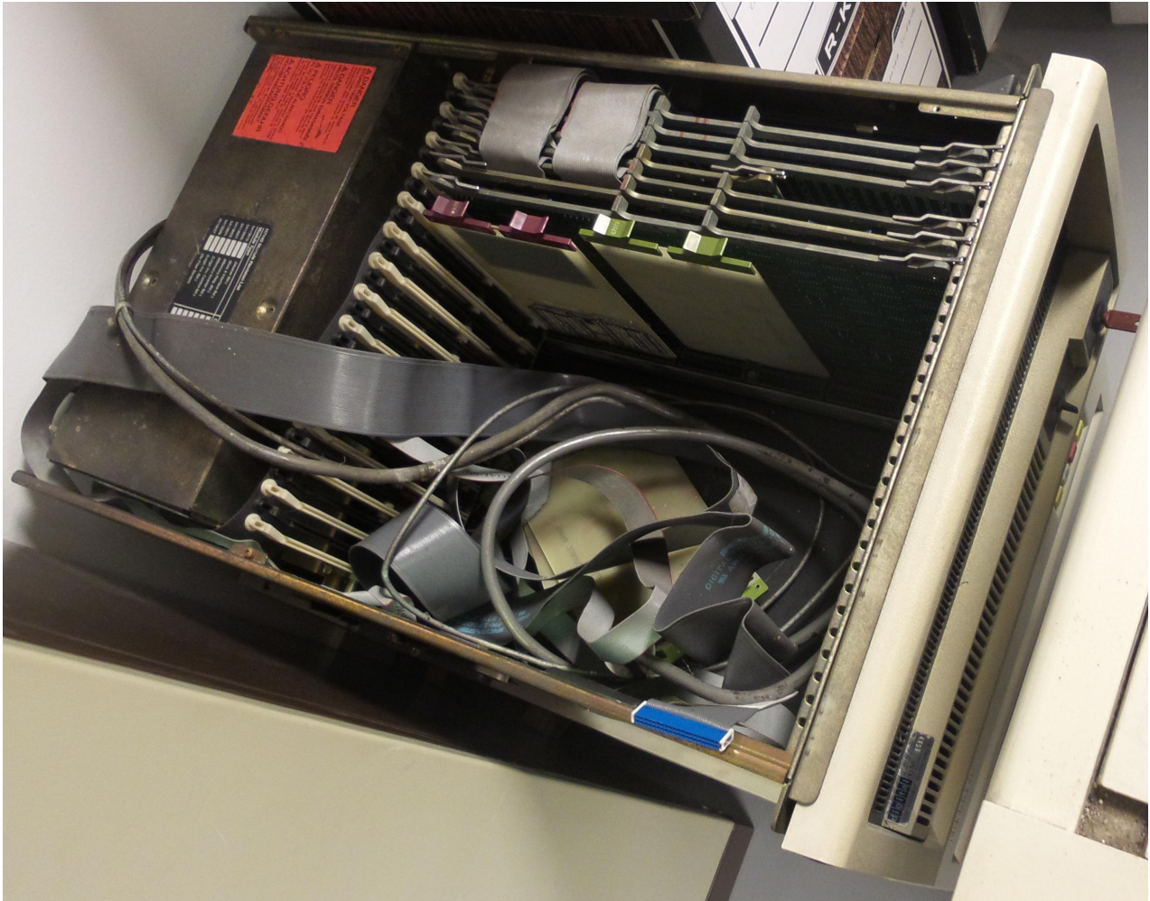
Figure 5: DEC PDP 11/24 CPU chassis, top three-quarter view
