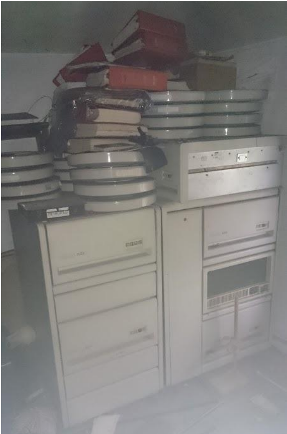
Figure 1: DEC PDP 11/24 system, disk cartridges and documentation in Boyle The unit at top right is an RL01 disk drive from TCD Library's PDP 11/34 (see elsewhere in this catalog)
