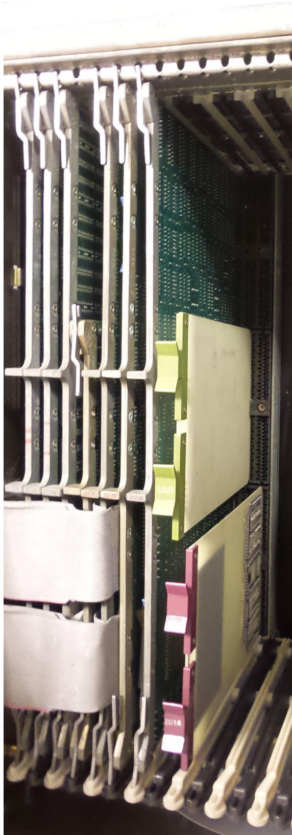
Figure 9: DEC PDP 11/24 CPU chassis Unibus modules
