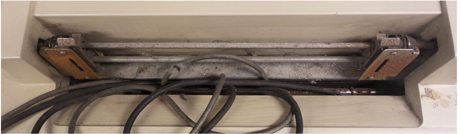
Figure 23: DEC LA36 DECwriter tractor-feed mechanism
