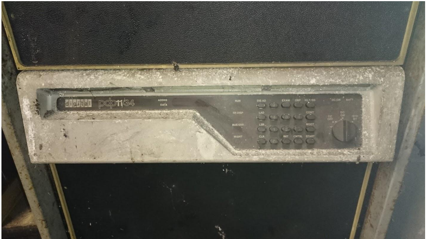
Figure 10: DEC PDP 11/34 in Boyle, front panel, note corrosion
