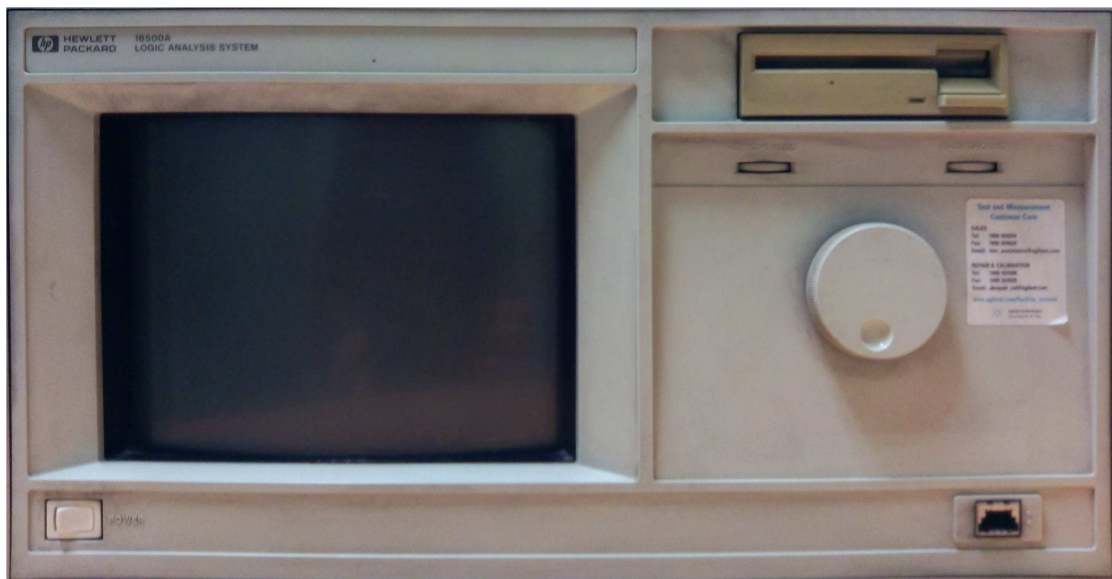
Figure 2: HP16500A front view, the connector at lower right is for a mouse, the controls below the floppy disk drive are for brightness (left) and ??? (right)
