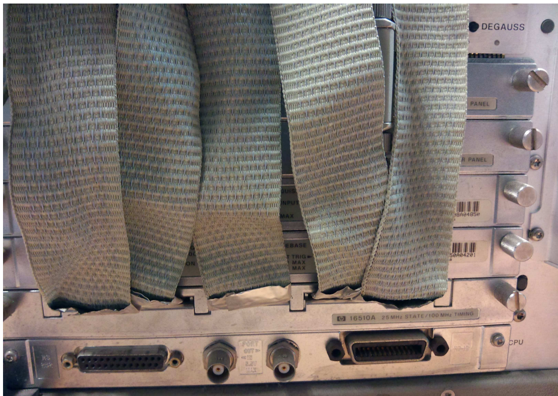
Figure 5: HP16500A 400Megasamples/sec digitizing oscilloscope modules: HP16531A digitizing oscilloscope acquisition, S/N: 2808A04850 HP16530A digitizing oscilloscope timebase, S/N: 2650A04201
