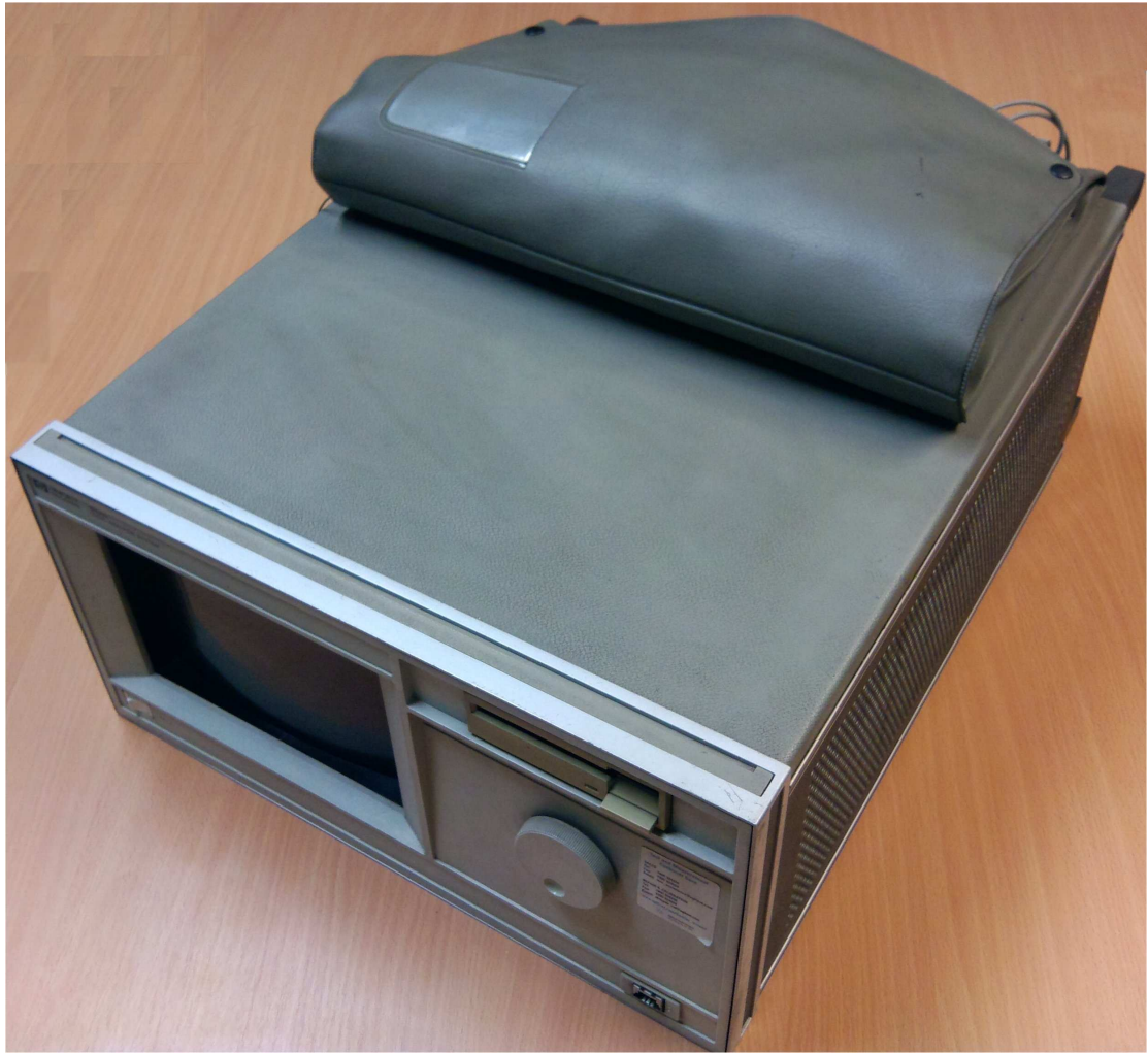
Figure 1: HP16500A front three-quarter view
