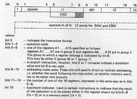
This type of instruction may be followed by a data word (16 bits) containing an address (m) or a positive or negative value. In the case of an address, bit 15 is not significant, except for character handling instructions.
