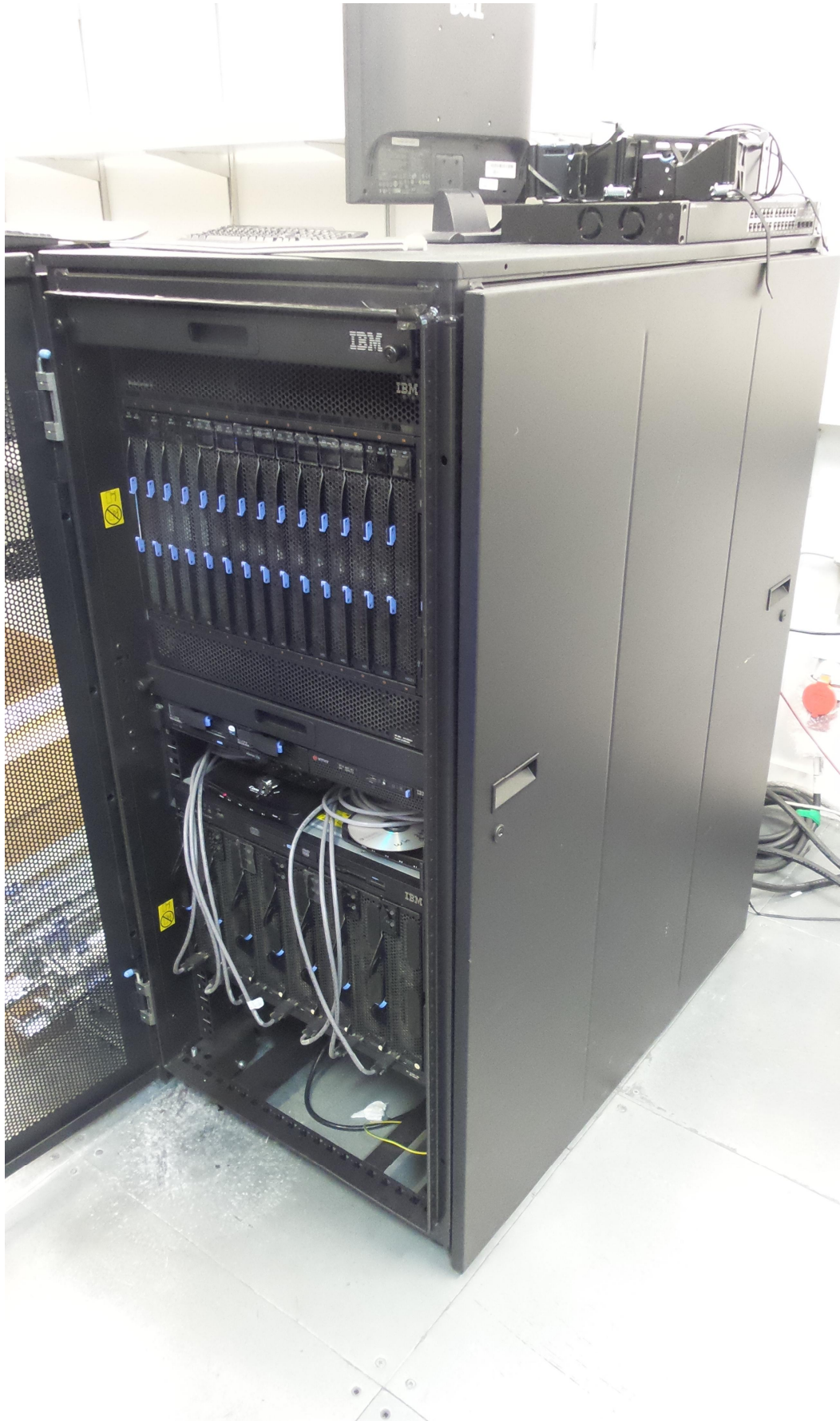
Figure 1: IBM BladeCenter QS20 three-quarter front view
