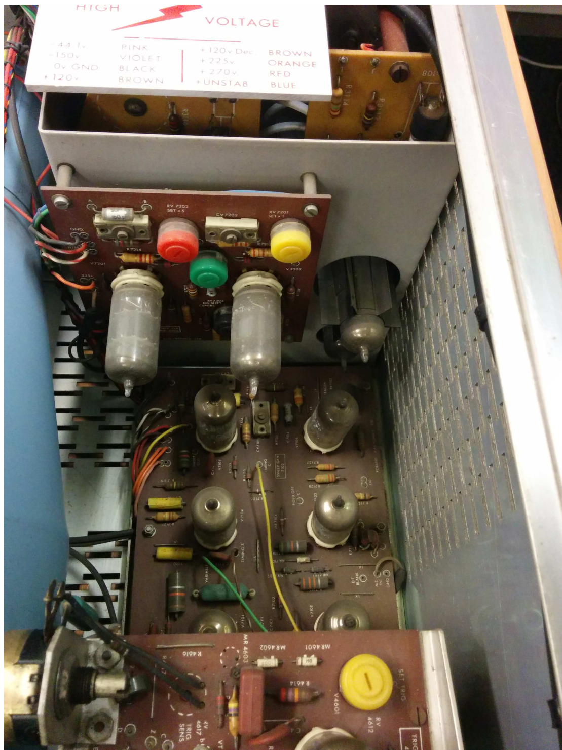
Figure 11: Roband RO50A MkII Oscilloscope X-axis circuits bottom: trigger circuit, middle: timebase (sweep) circuit, top: X-axis output circuit
