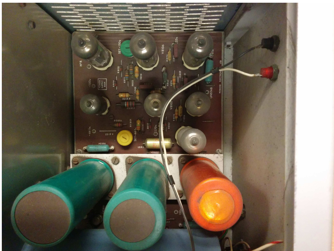
Figure 8: Roband RO50A MkII Oscilloscope rear right top internal view Power supply circuit (for -44.1V, -150V, +225V, +270V)
