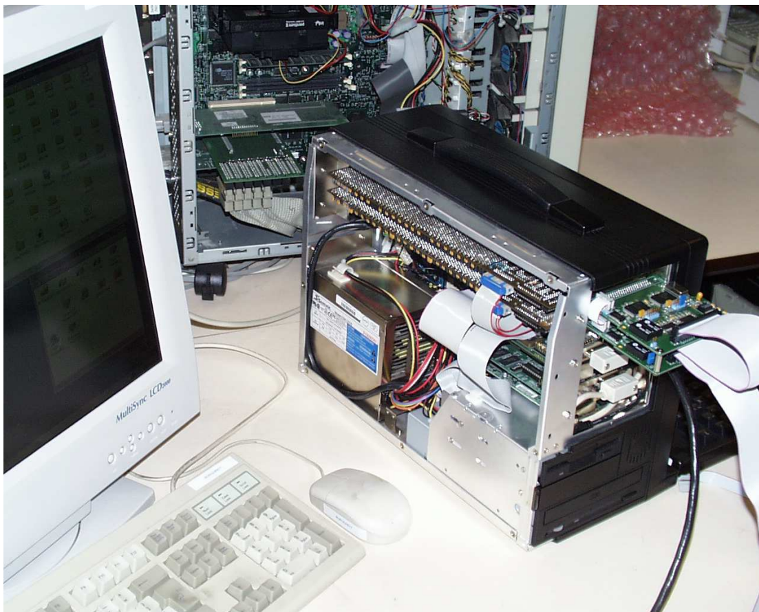
Figure 7: SCI Tracer in use for performance monitoring via Dolphin probe card
