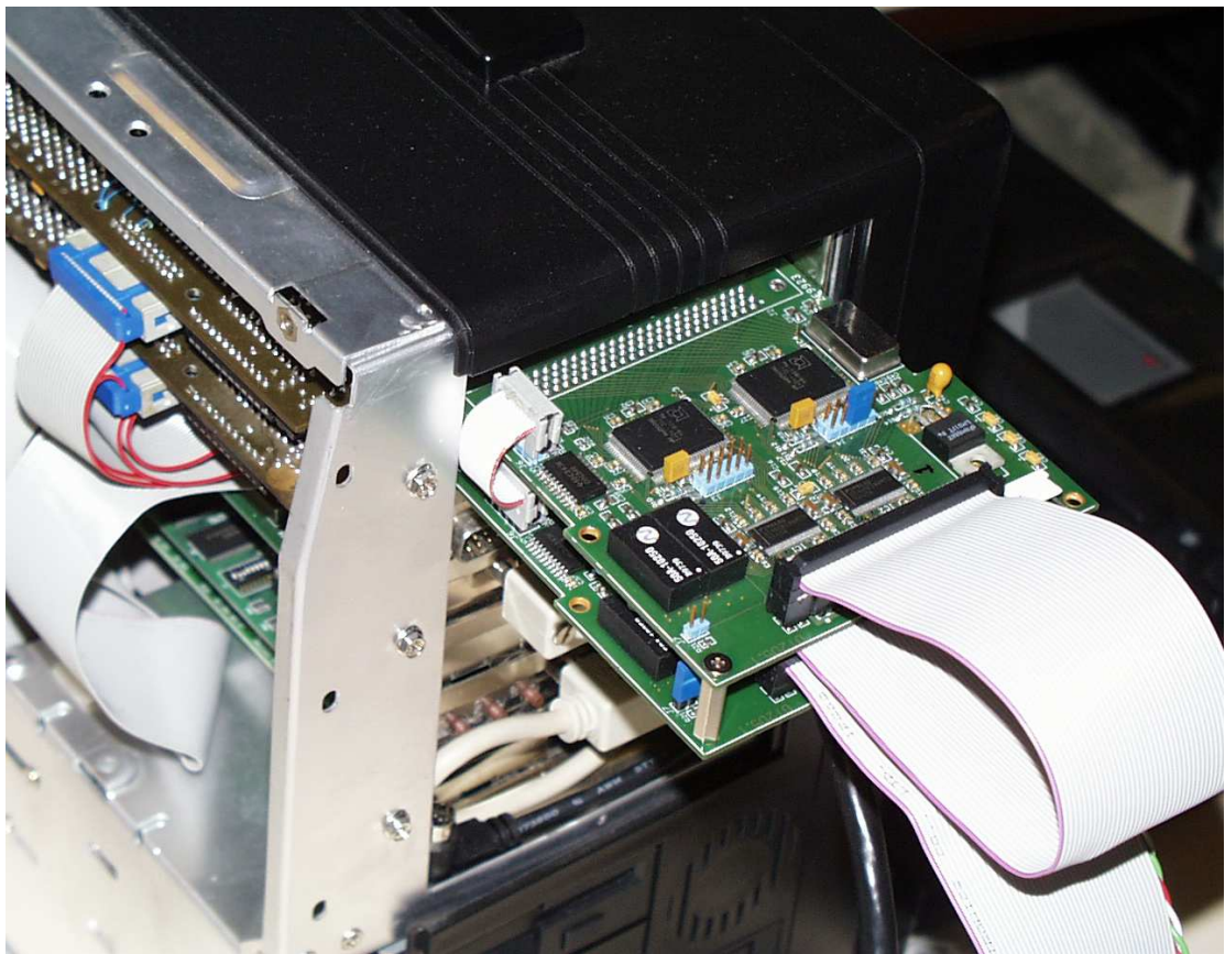
Figure 11: SCI Tracer connections to DT205.1 Probe Adapters
