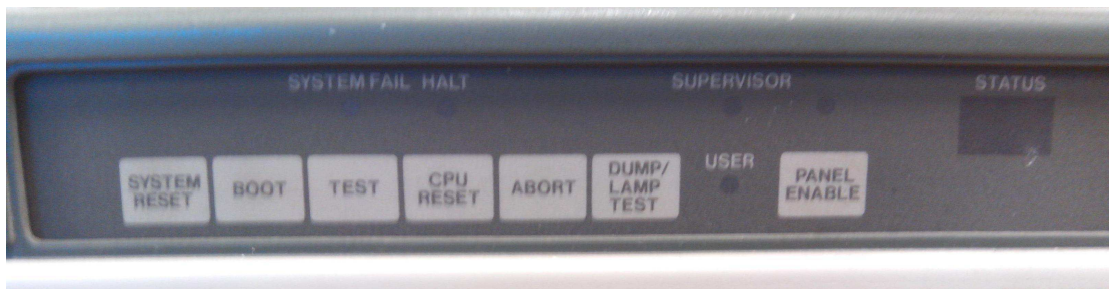
Figure 5: SORD M685 control panel
