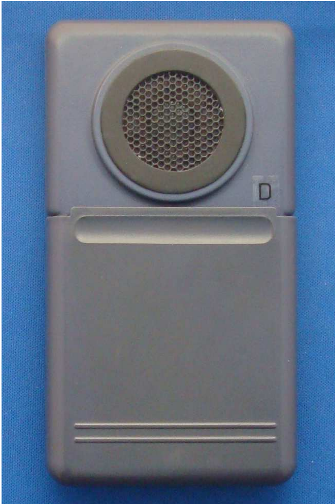
Figure 2: Texas Instruments Pocket Dialer rear view To use, the speaker is faced towards the telephone microphone
