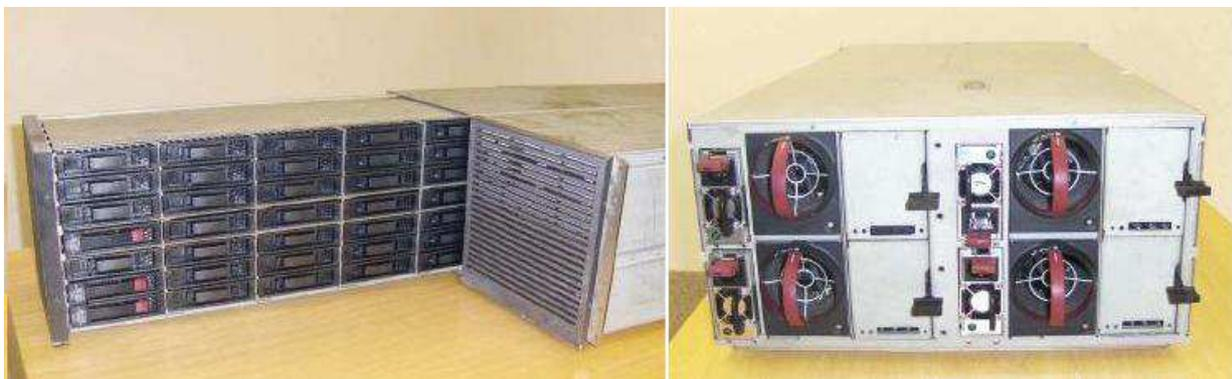
Figure 5: HP ExDS storage chassis, front and rear views
