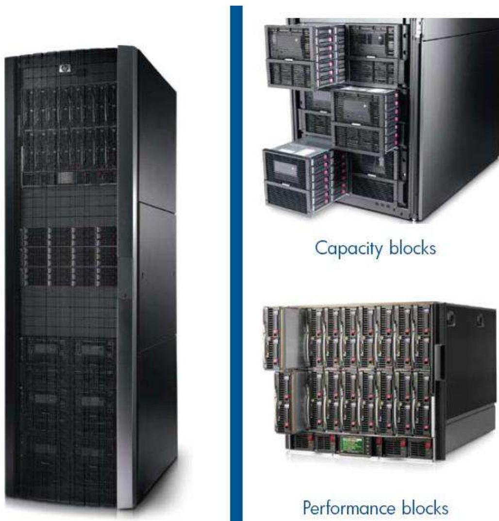
Figure 1: HP ExDS system and constituent blocks, three-quarter views (courtesy HP)
