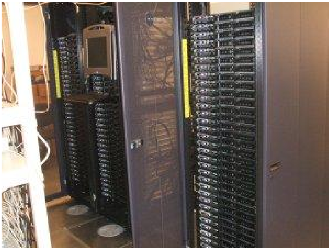
Figure 2: csTCDie 96-node Beowulf Cluster Racks
