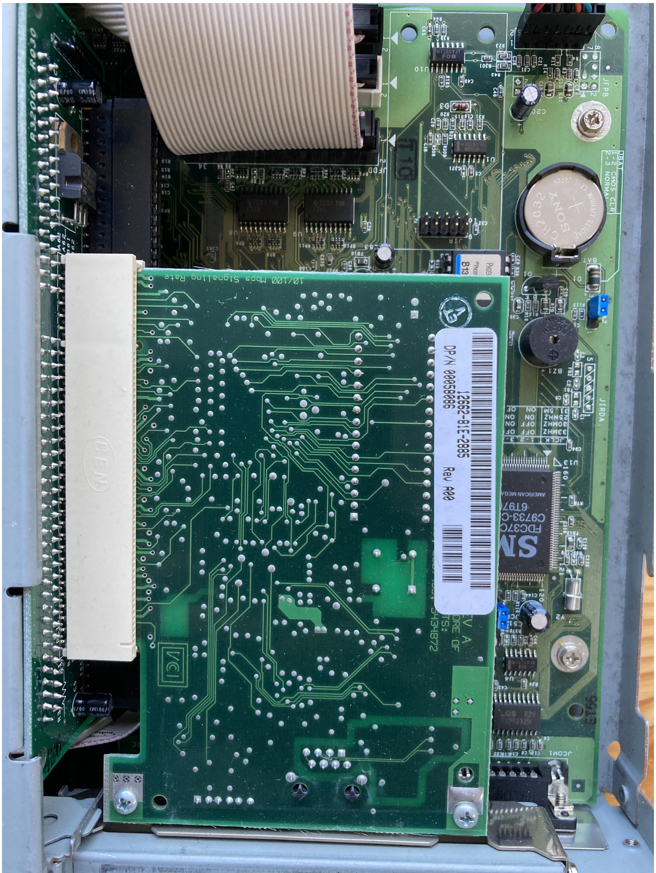
Figure 8: csTCDie Beowulf Cluster NIS server, internal view, Ethernet adapter
