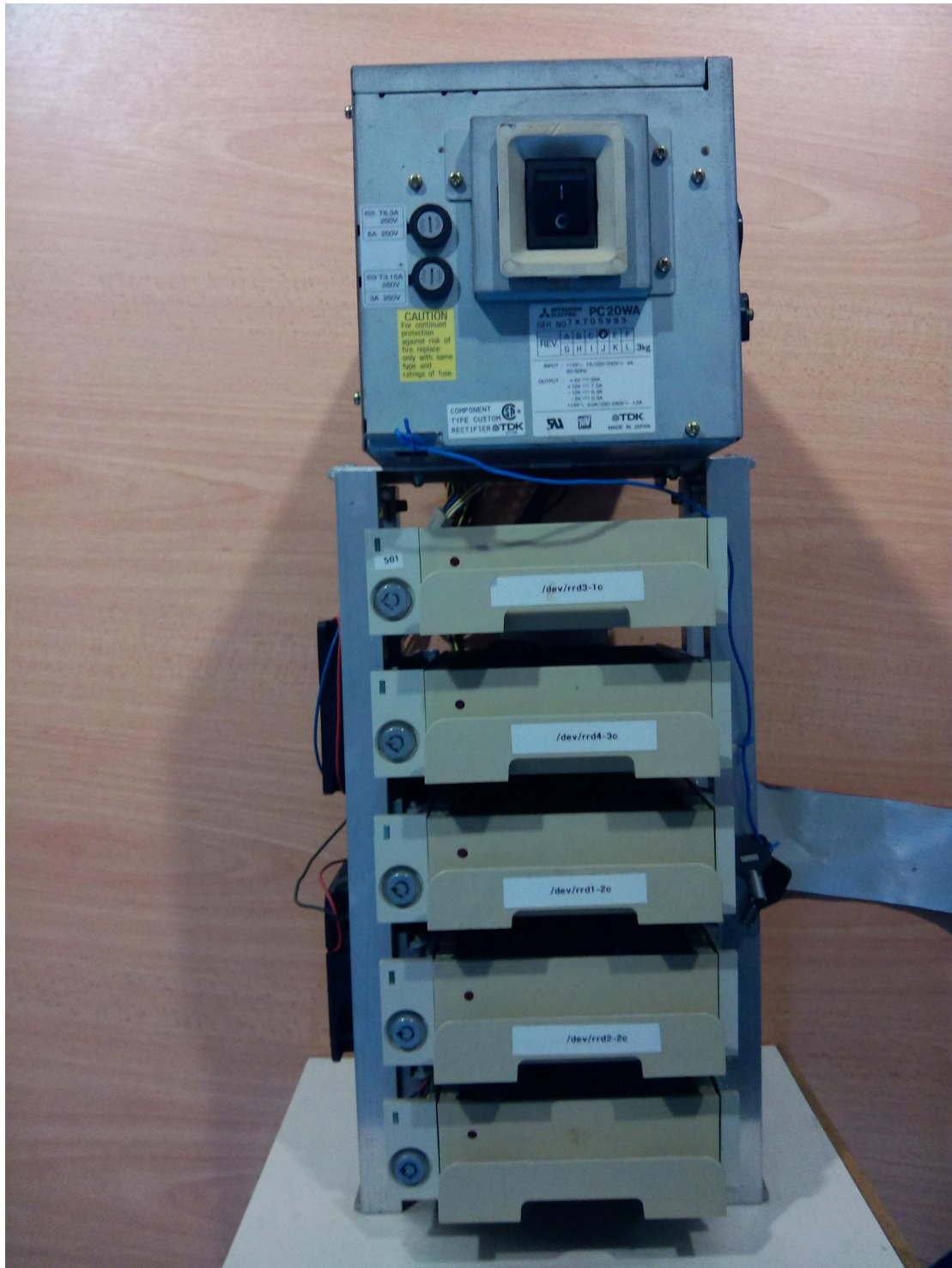
Figure 17: csTCDie Beowulf Cluster NIS server, RAID array TCD-SCSS-T.20150217.003
