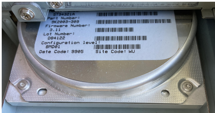
Figure 13: csTCDie Beowulf Cluster NIS server, internal view, hard disk identification Seagate ST34321A 4.3GB IDE hard disk, 5 heads, 17 sectors of 512 bytes, 33344 cylinders
