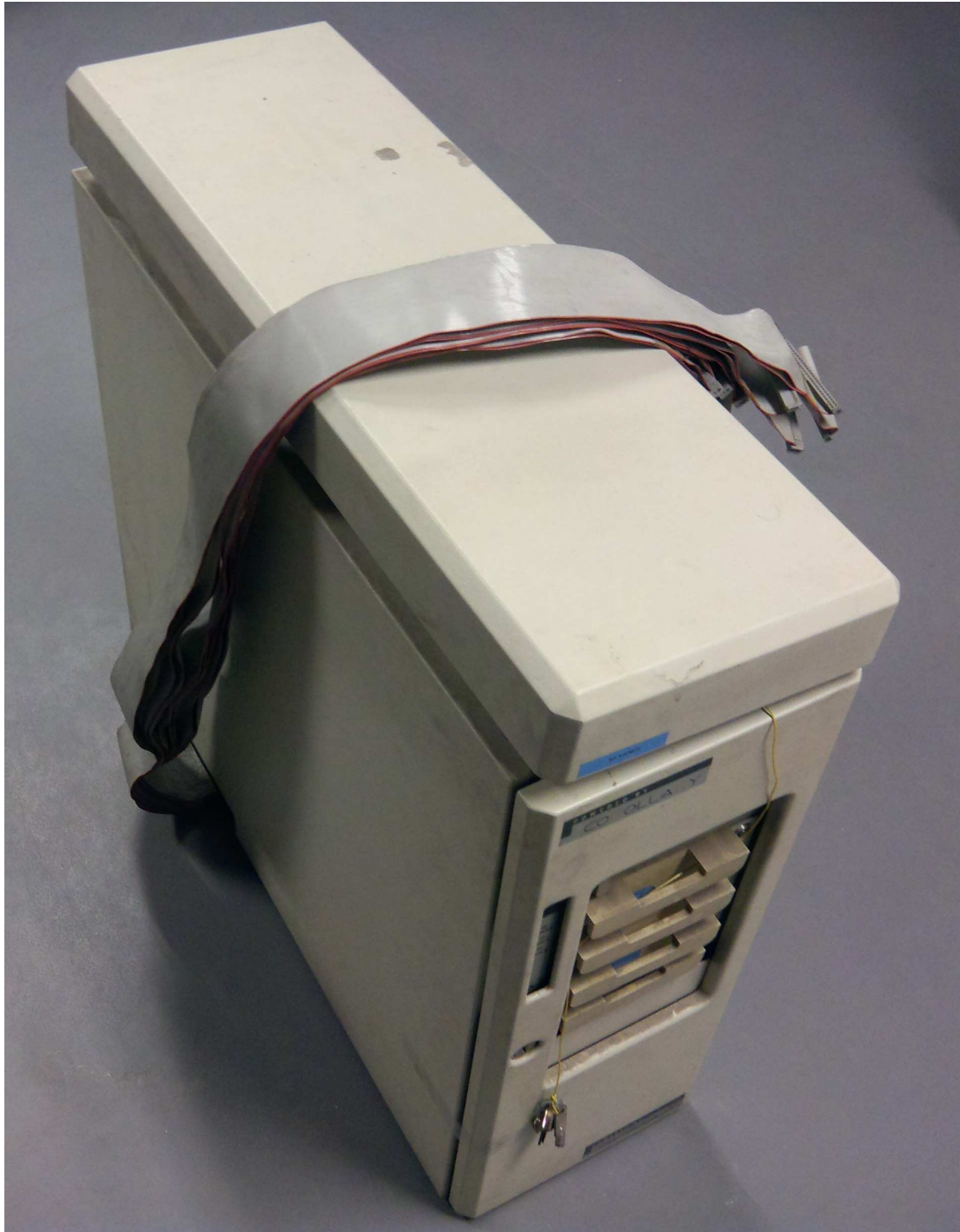
Figure 1: Corollary XM front three-quarter view Cables are Stable Disk connections to external RAID chassis
