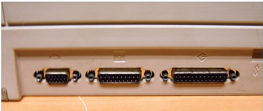
Figure 7: Apple Macintosh M5126 left rear closeup DB-15 video adapter, DB-19 external floppy disk, DB-25 SCSI
