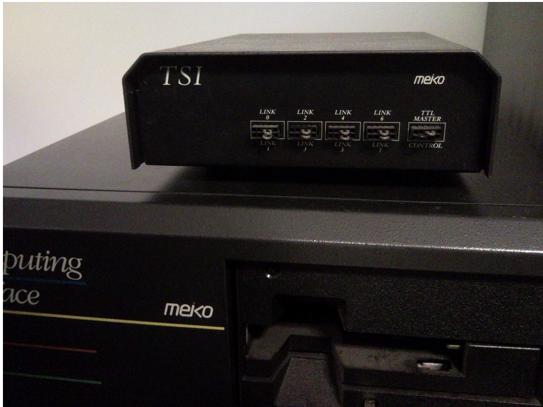
Figure 2: Meiko CSI Computing Surface link extender closeup
