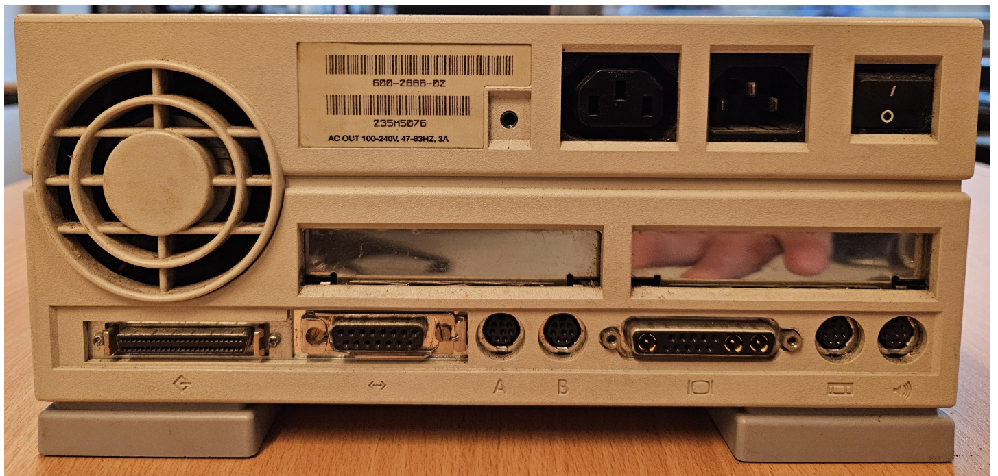
Figure 6: Sun Sparcstation IPX, S/N: 600-2886-02 235M5076, rear closeup.
