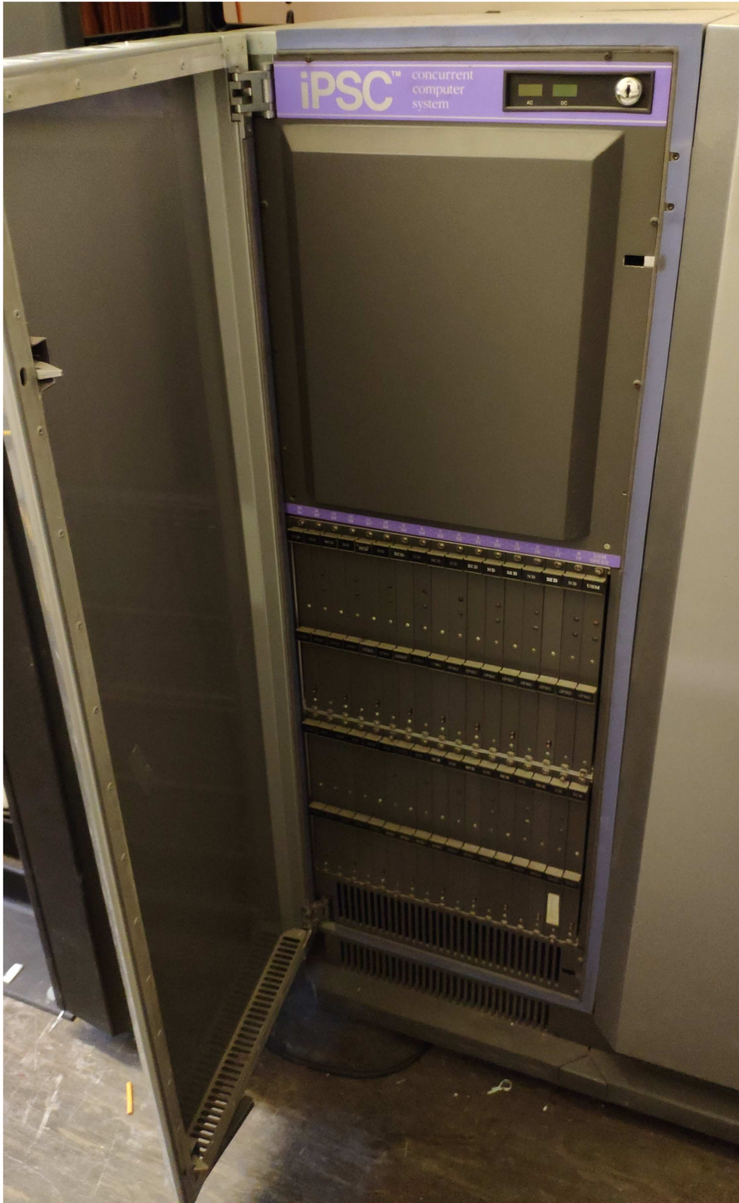
Figure 3: Intel iPSC Hypercube left rack front three-quarter view Photograph courtesy Tom Kearney
