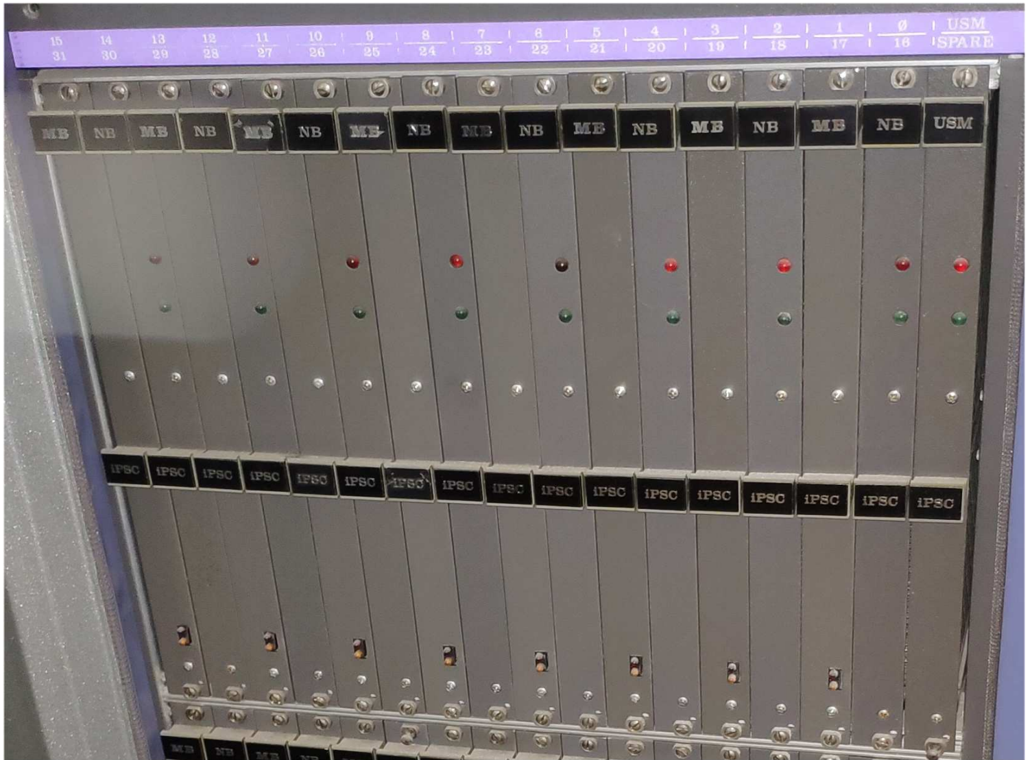
Figure 5: Intel iPSC Hypercube left rack upper blade chassis Photograph courtesy Tom Kearney
