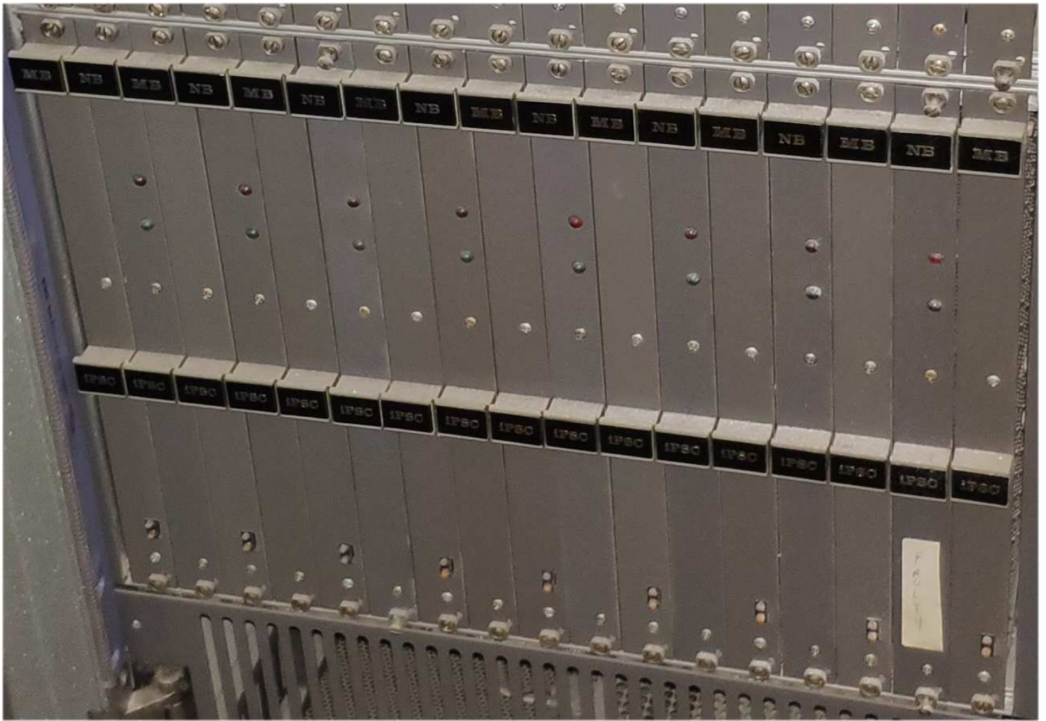
Figure 6: Intel iPSC Hypercube left rack lower blade chassis Photograph courtesy Tom Kearney
