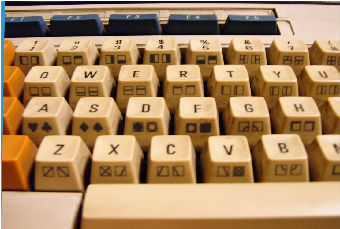
Figure 3: Sharp MZ-711(1) left-side keyboard key front markings closeup
