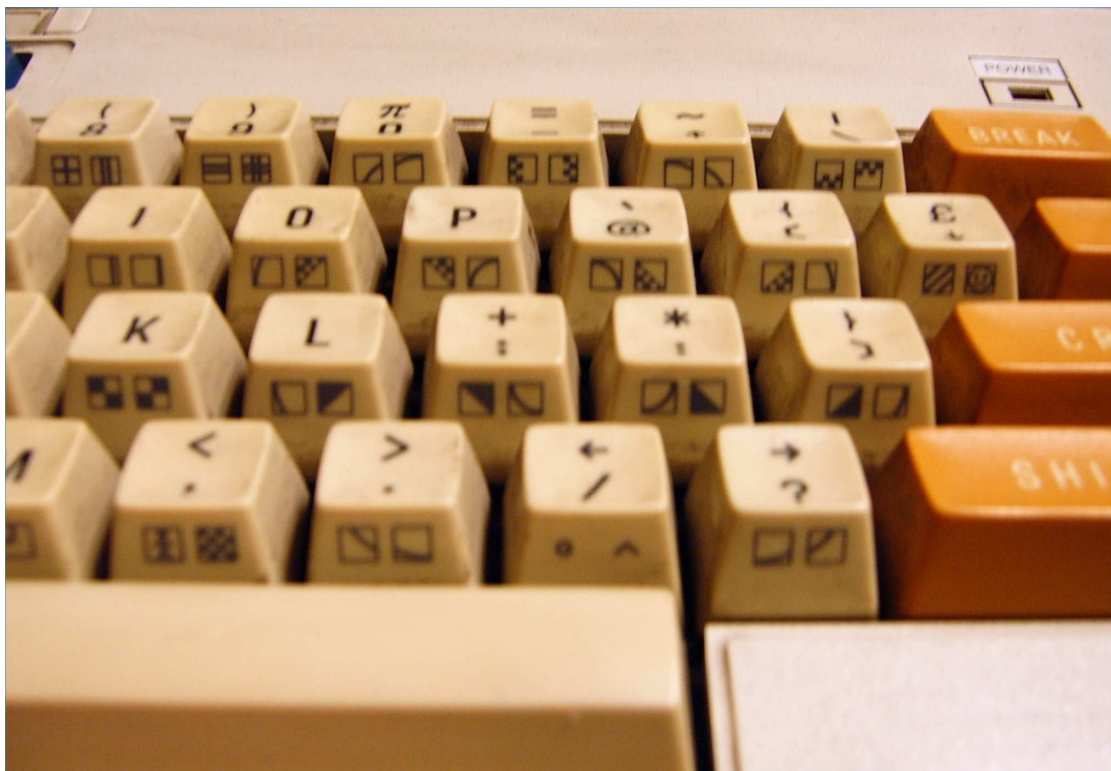
Figure 4: Sharp MZ-711(1) right-side keyboard key front markings closeup
