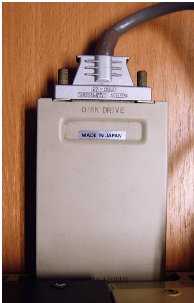
Figure 9: Sharp MZ-711(1) I/O Bus Quickdisk Interface top view
