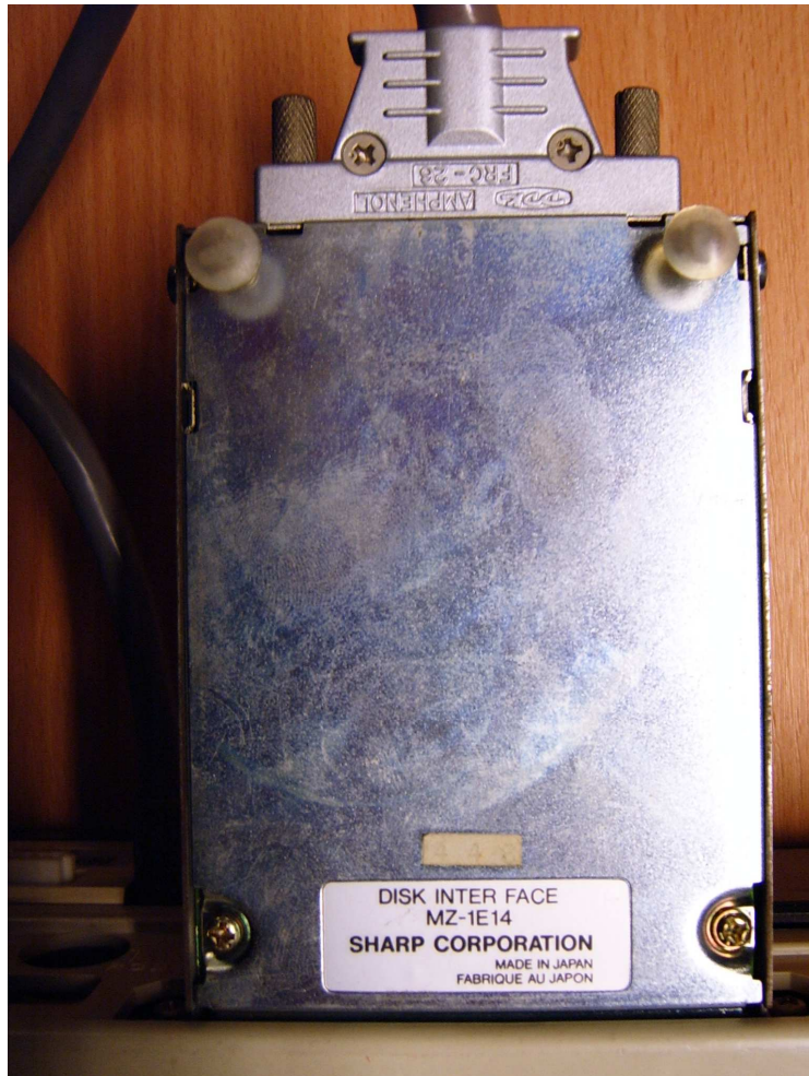
Figure 10: Sharp MZ-711(1) I/O Bus Quickdisk Interface bottom view Model: MZ-1E14, S/N: 440
