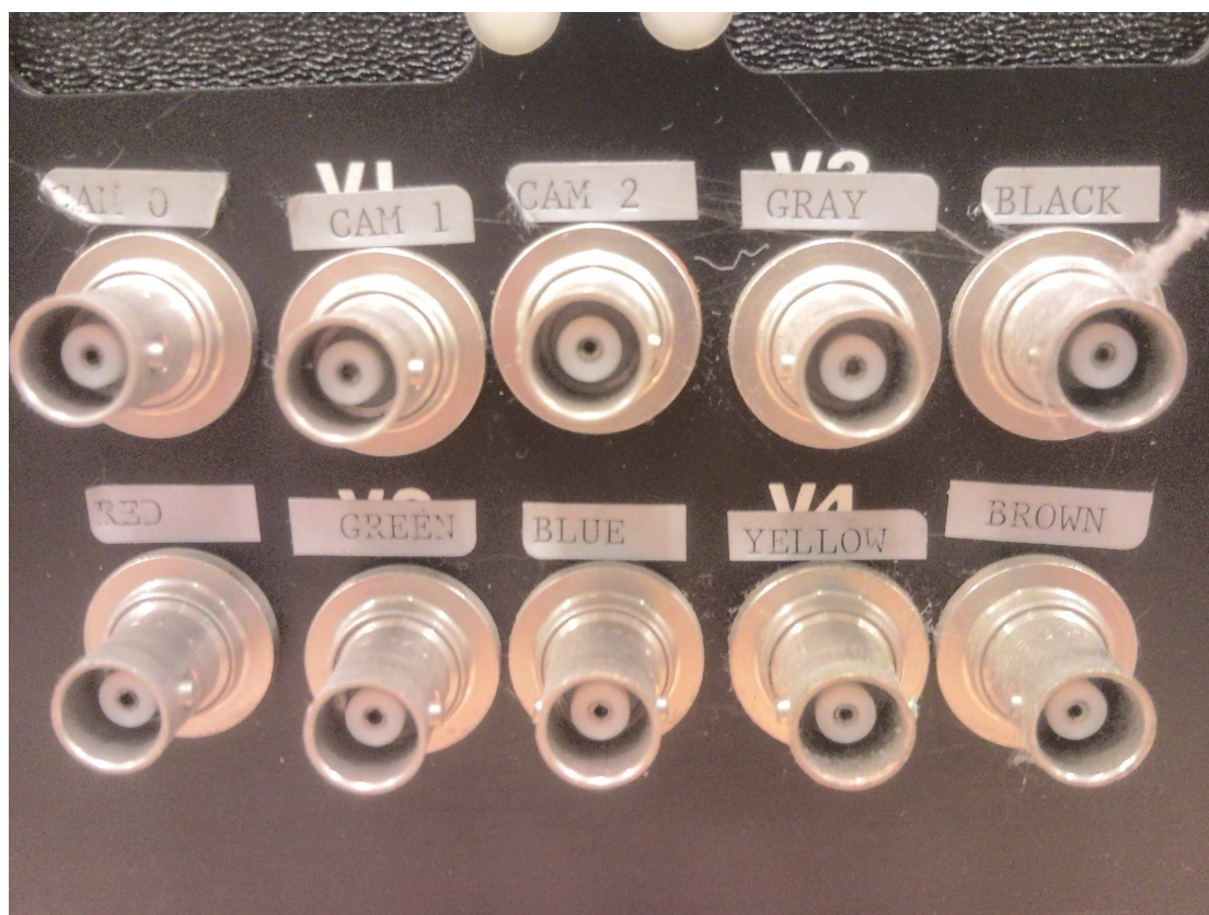
Figure 7: Heurikon HSE-10R rear BNC video connectors CAM 0, CAM 1, CAM 2, GRAY, BLACK RED, GREEN, BLUE, YELLOW, BROWN
