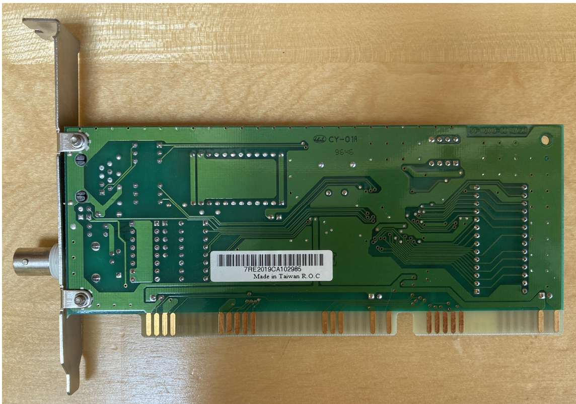
Figure 14: Unidentified Combi (Coax+RJ45) Ethernet ISA Card, uses RTL8019, labelled CY-01A, bottom view TCD-SCSS-T.20121208.046.04
