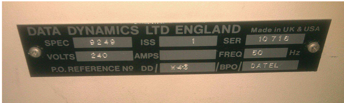
Figure 11: Teletype Model 43 manufacturing label Manufactured by Data Dynamics Ltd Spec: 9249, ISS: 1, S/N: 10716 Volts: 240, Amps: -, Freq: 50 Hz P.O.Reference No: M43, BPO: DATEL
