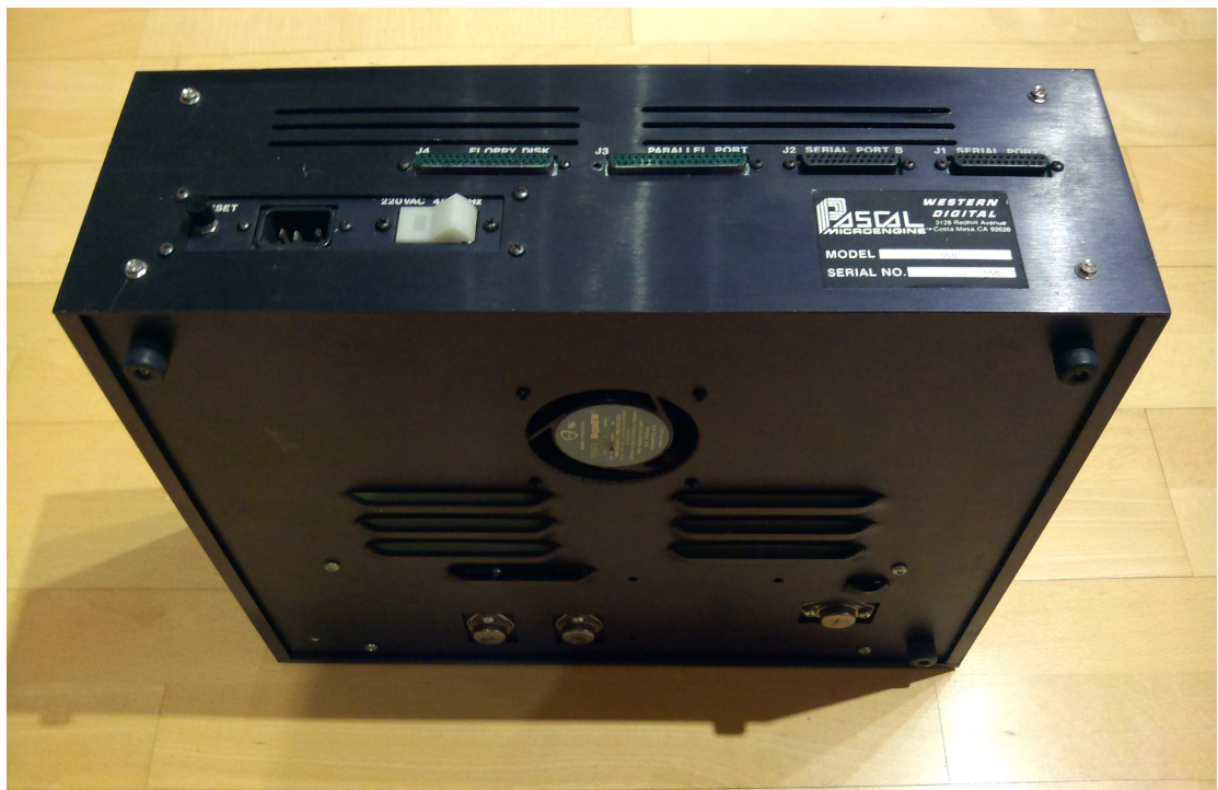
Figure 6: WD90 Pascal Microengine bottom view, ventilation and power transistors
