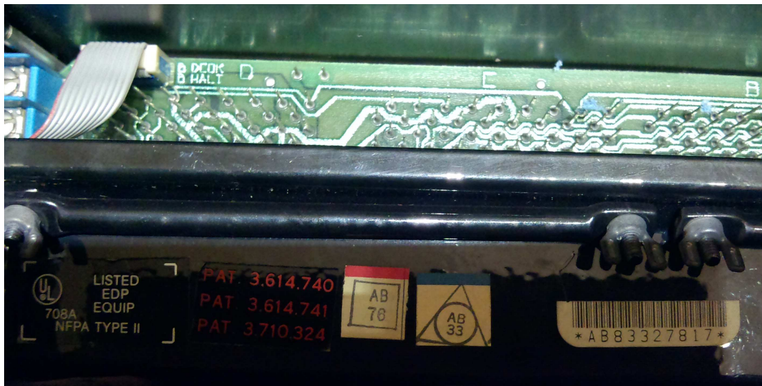
Figure 18: DEC VAX 11/780 Console Processor regulatory labels and serial number S/N: AB83327817
