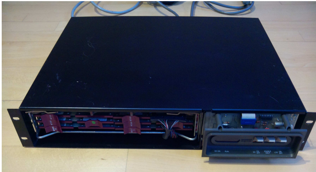
Figure 7: DEC VAX 11/780 Console Processor internal front view
