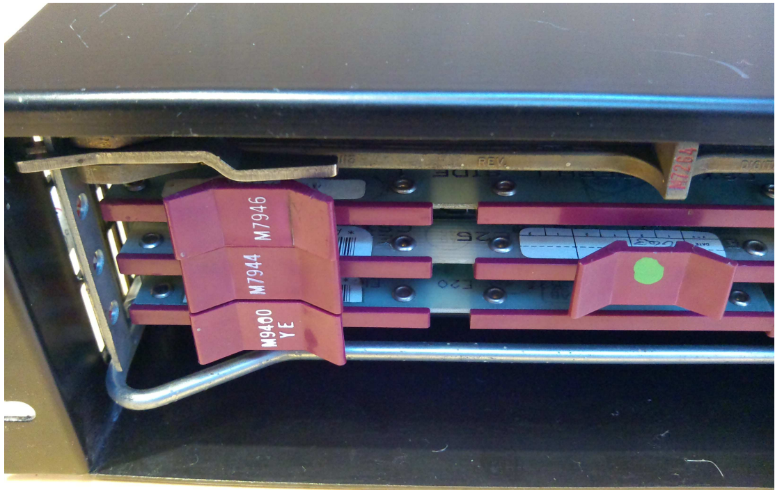
Figure 11: DEC VAX 11/780 Console Processor left Qbus boards M8460-YE, M7944, M7946, full-width CPU board at top
