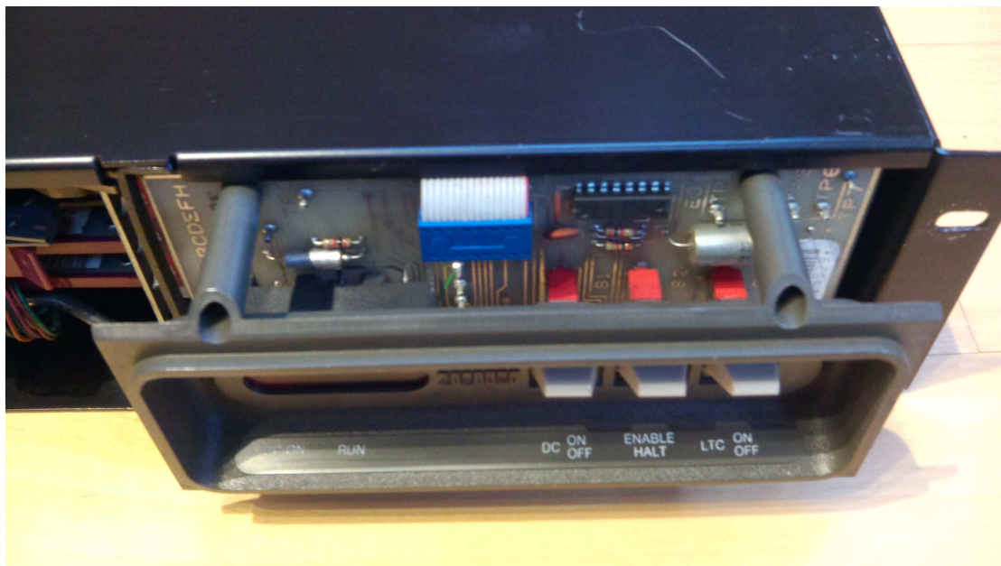
Figure 8: DEC VAX 11/780 Console Processor internal control panel view
