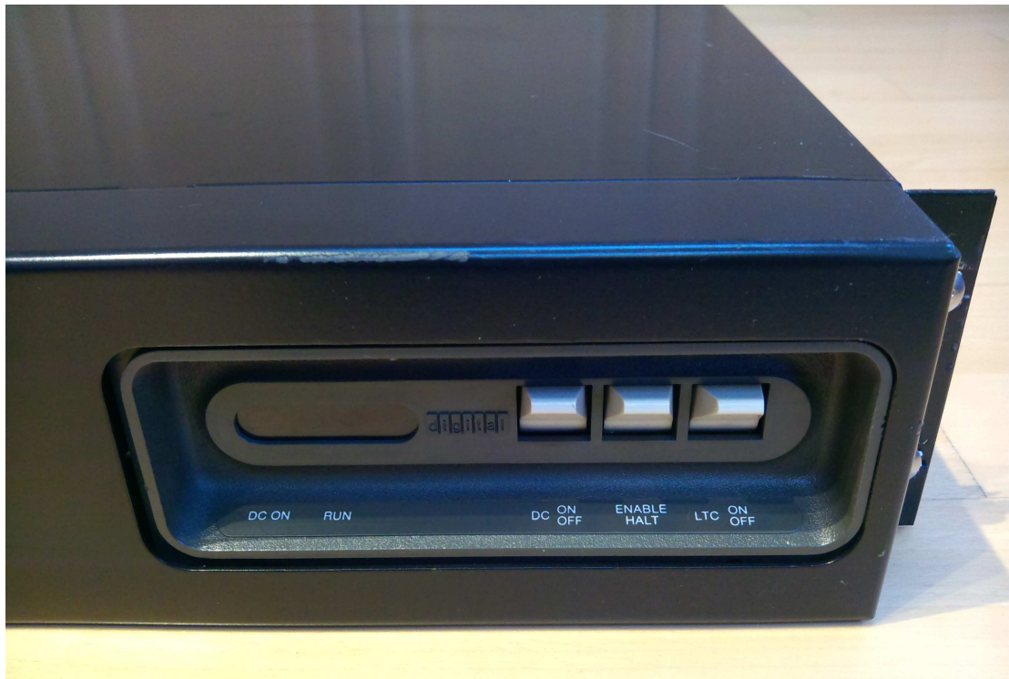
Figure 2: DEC VAX 11/780 Console Processor control panel
