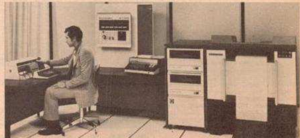
A basic configuration of the Burroughs B1712 includes the multipurpose card unit for 96-column cards, console typewriter, two disk cartridge drives and a line printer.
