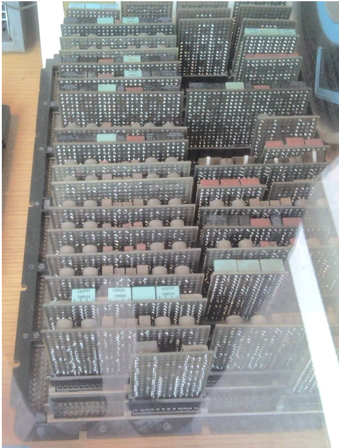
Figure 9: IBM 360/44 CPU logic chassis and hybrid logic modules
