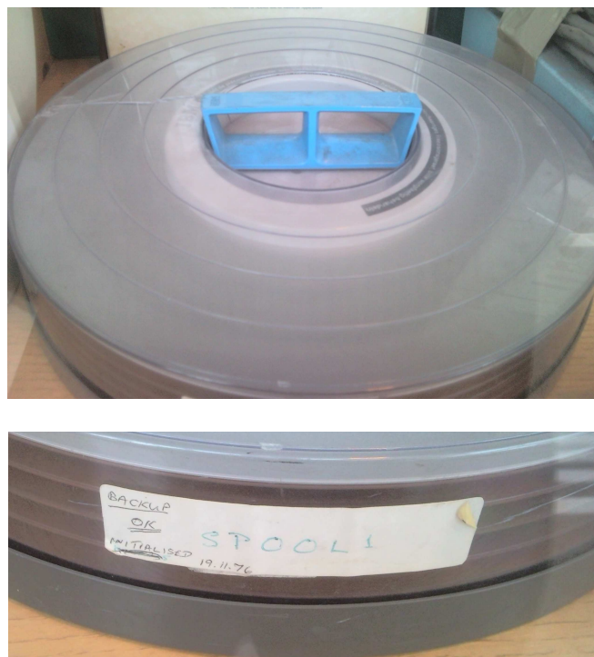
Figure 11: IBM 1316 7.25MB 14-inch Disk Pack for use on an IBM 2311 drive Marked 'Backup Spool 1 initialised 19.11.1976'
