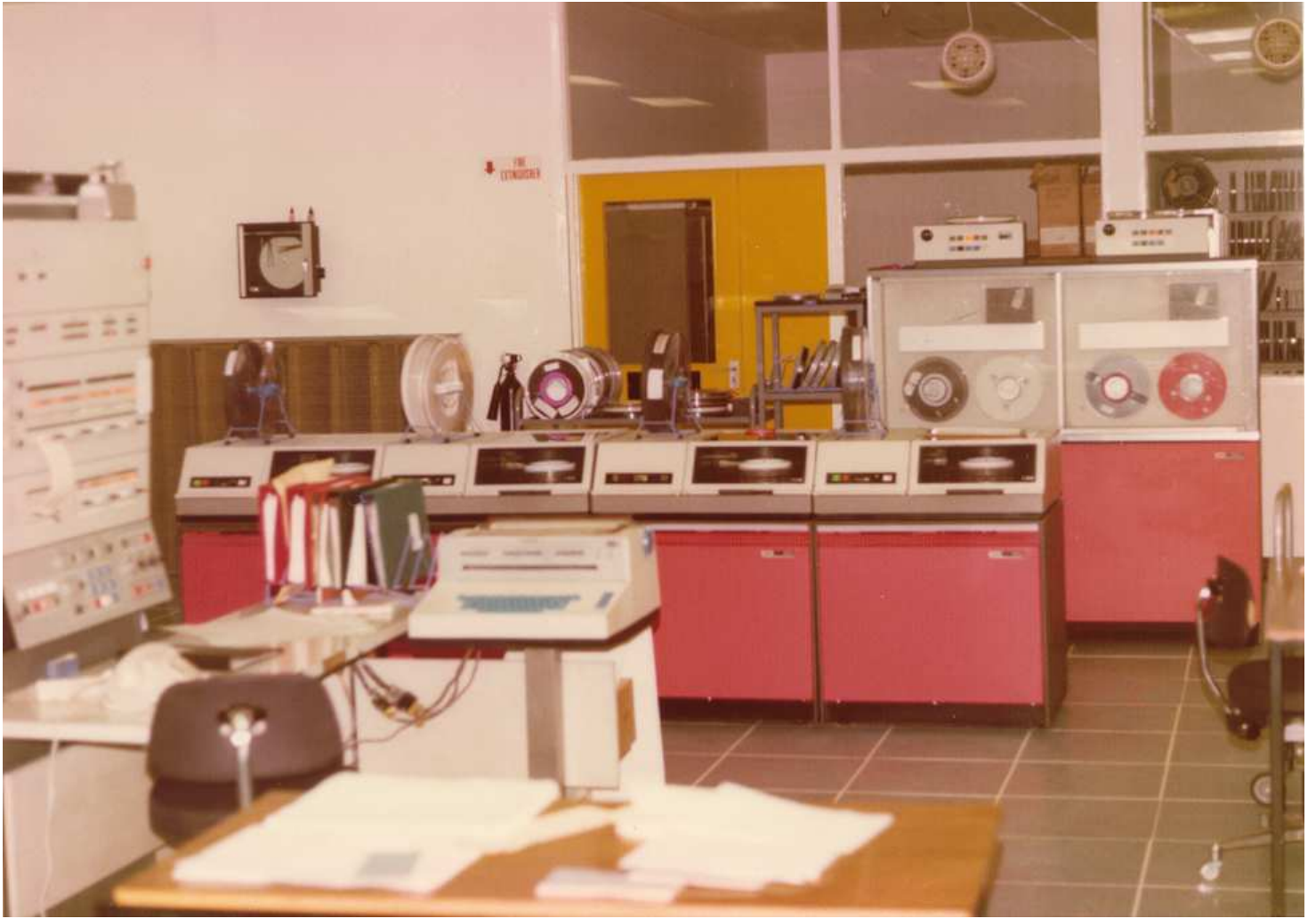
Figure 3: IBM 360/44 in action c.1976, image courtesy Mike Nowlan Console at left, IBM 1052 console printer/keyboard in foreground 4 x IBM 2311 7.25MB disk drives, 2 x IBM 2400 magtape drives at rear
