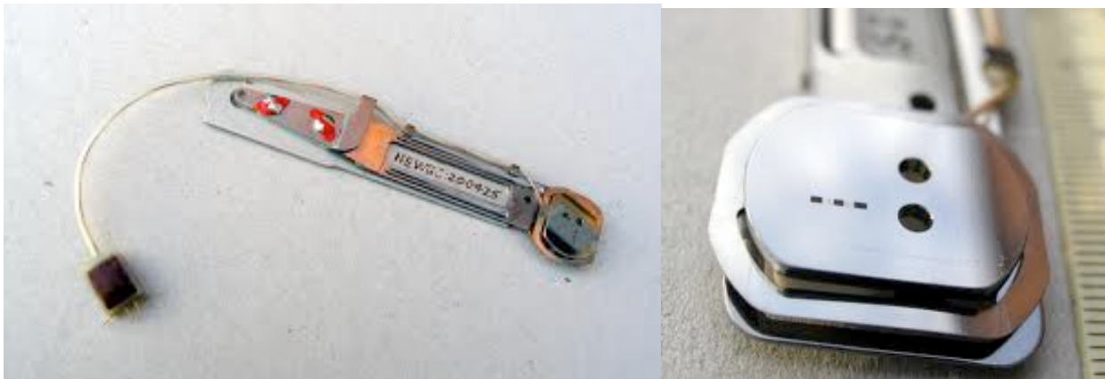
IBM 2311 Flying Head Assembly (Ref 6)
