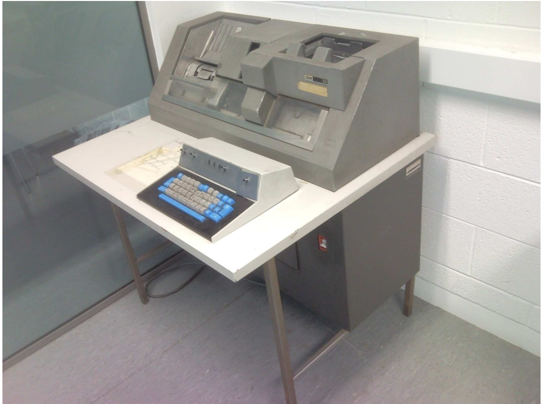
Figure 1: IBM Card Punch Model 29C three-quarter view
