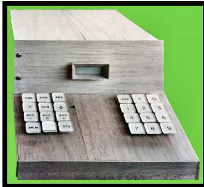
Osborne housed his prototype calculator in a case made of balsa wood and Elmer's glue, which he then painted a metallic green selected from the 1960s paint palette of GM's Cadillac automotive division.
