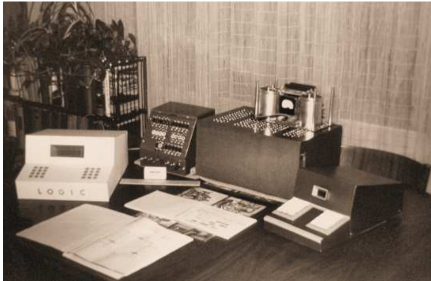
Tom Osborne demonstrated his calculator to several companies in his apartment, where he'd built the machine. Here, the calculator prototype (right) is readied for the showing, along with the logic module (center box), the power supply (on top of the logic module), and a specialized tester Osborne built (to the left of the logic module) that allowed him to debug the prototype without the expensive test equipment he'd otherwise need for such a project. The white mockup calculator on the left shows how large Osborne expected a finished calculator to be, once it housed the logic and power supply in addition to the keyboard and display.
