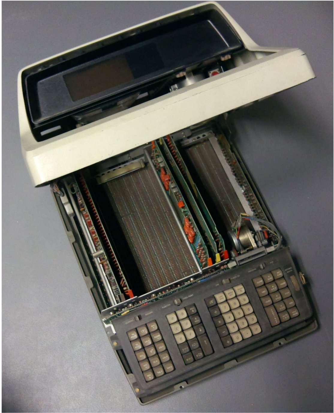
Figure 4: HP9100A internal view with top lifted
