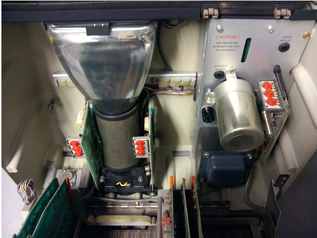
Figure 5: HP9100A CRT display and power supply
