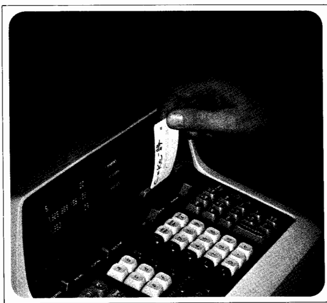
Fig. 8. Programs can be entered into the calculator by means of the magnetic program card. The card is inserted into the slot and the ENTER button pressed.
