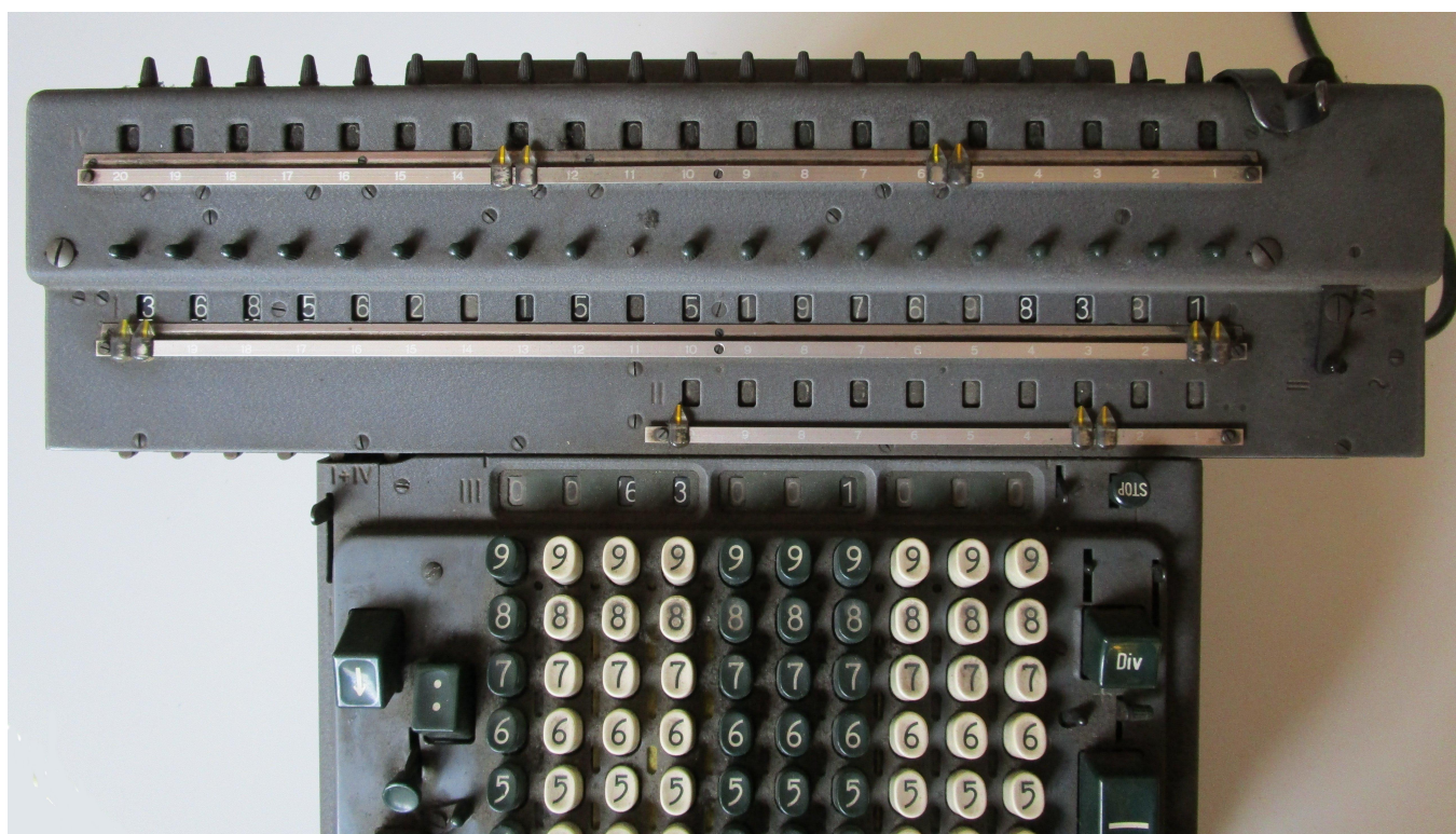
Figure 3: MADAS 20BTZG Calculator carriage Note accumulator product Register I and accumulator Register IV twirlers
