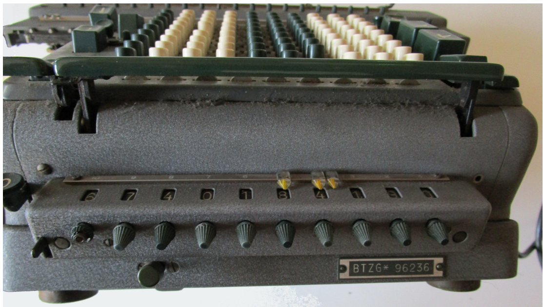
Figure 5: MADAS 20BTZG Calculator lower front closeup showing multiplier twirlers and controls
