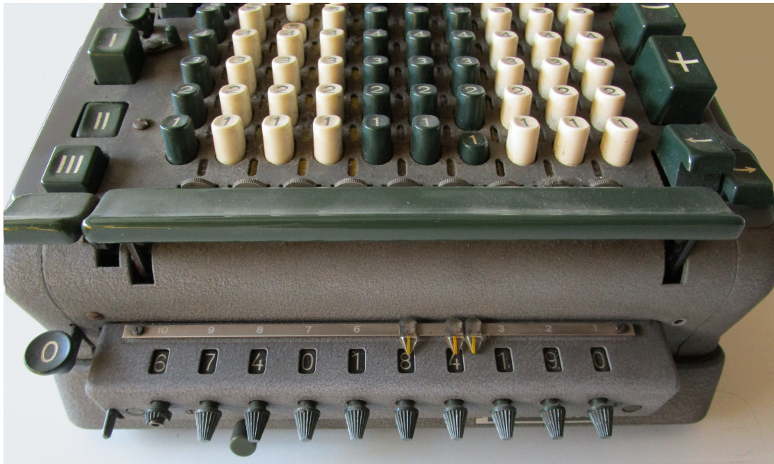
Figure 4: MADAS 20BTZG Calculator lower front closeup showing multiplier Register 0
