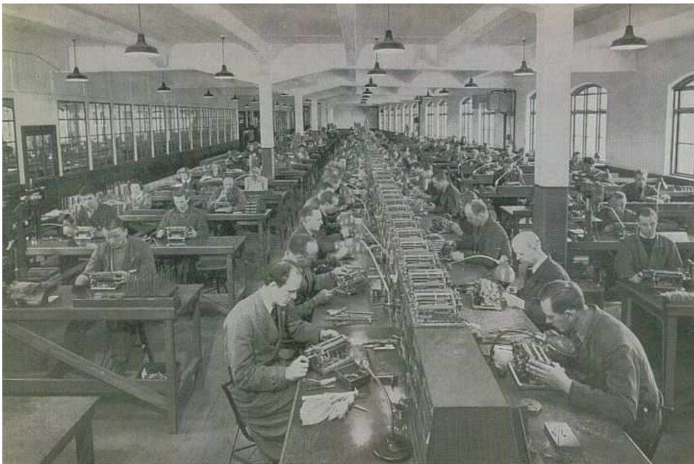
Production of Facit ESA-0 (around 1954) - This model consists of about 2200 items!
