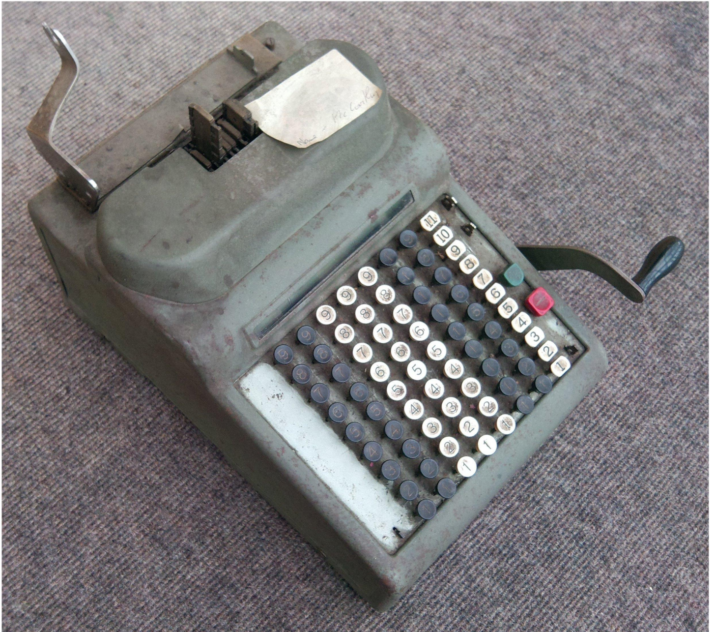
Figure 1: R.C.Allen Model 8s Calculator three-quarter view
